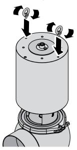
Once valve installation has been completed, remove the eyebolts and put the screws back in.
