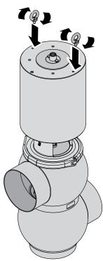
Once valve installation has been completed, remove the eyebolts and put the screws back in.
