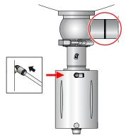
Weld it care/ try to make a stressless welding to avoid deformatin on sealing areas. Check the valve for regular operation after welding
