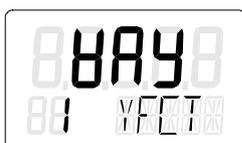
2. Use the
