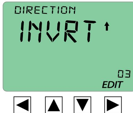
If using a Normally Open or Normally Open Double Acting valve it is correct to use this parameter (INVRT).
