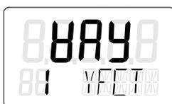
2. Set the "YFCT" parameter to "turn". To do this, press
