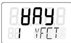
2. Call the "2.YAGL" parameter. To do this, briefly press the
