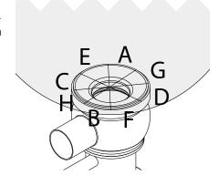
Assemble the valve after welding.
